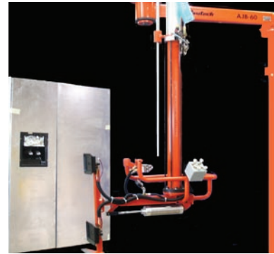
Pedestal mounted AJB with Vertical Lift Cylinder handling white goods.
