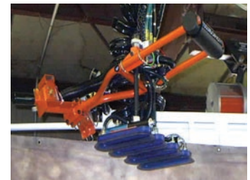
Hook hung vacuum end-effector with extended pivoting handle.
