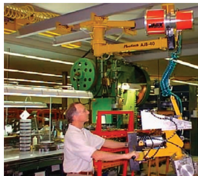
Trolley mounted AJB with balancer handling a bearing race.
